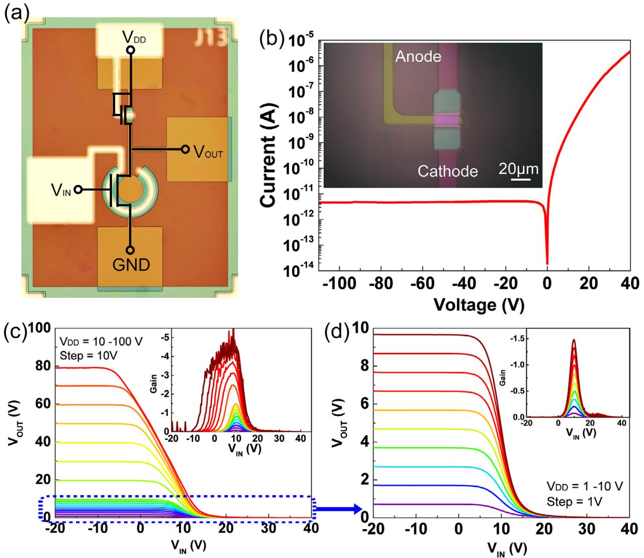
**Figure 5.** (a) Structure diagram of an HV inverter which is composed of an HVTFT drive and an HVD load. (b)  $I$ - $V$  characteristics of HVD with rectification ratio of  $\sim 10^6$  and  $V_{BR}$  more than 110 V. (c) Voltage-transfer characteristics of the HV inverter with a maximum operation voltage of 80 V. Inset is the voltage gain. (d) Low-voltage operation of the HV inverter down to 1 V. Inset is the voltage gain.
